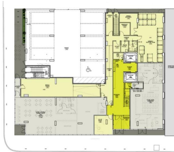
1:200 Ground Floor Plan Support and Service Space Residential Lobby Restaurant and Training Facility
