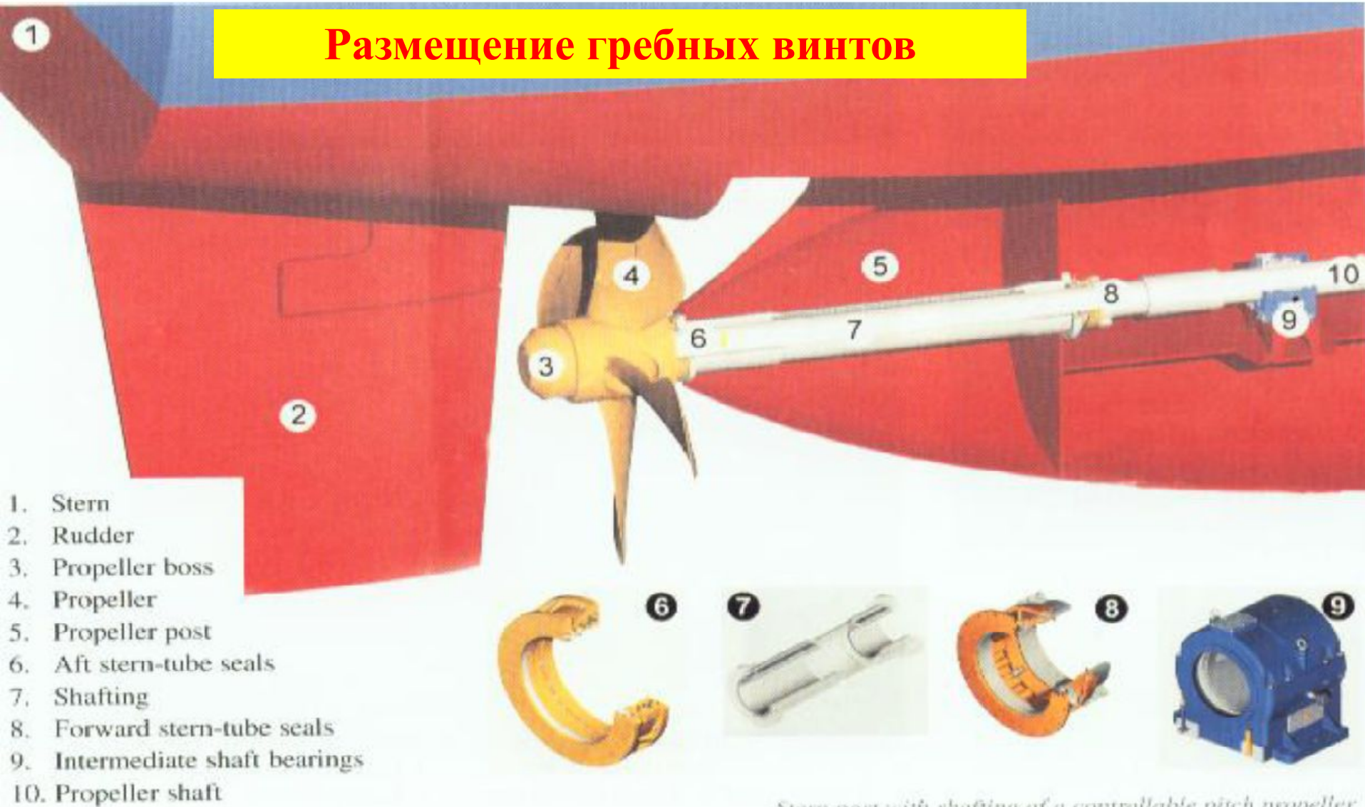
Stern post with shafting of a controllable pitch propeller
