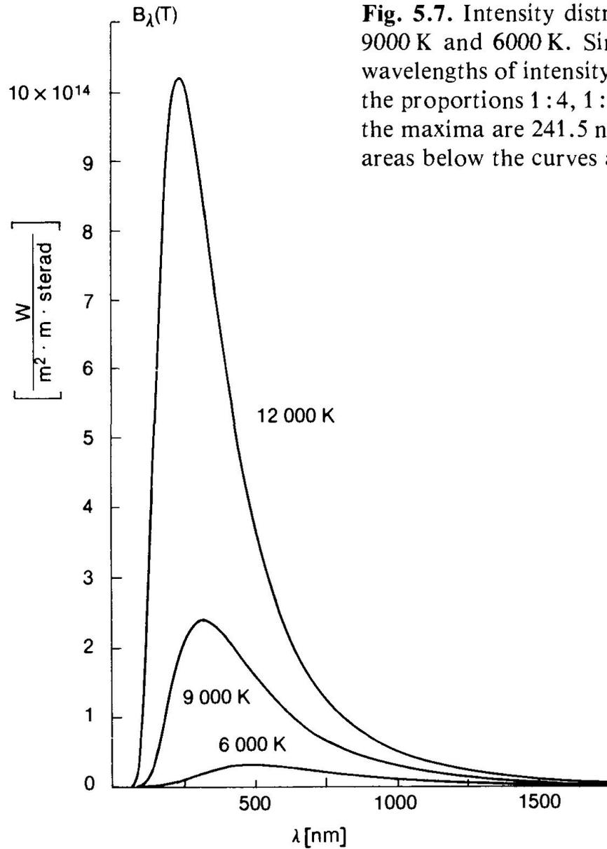
**Fig. 5.7.** Intensity distributions of blackbodies at temperatures 12 000 K, 9 000 K and 6 000 K. Since the ratios of the temperatures are 4:3:2, the wavelengths of intensity maxima given by the Wien displacement law are in the proportions 1:4, 1:3 and 1:2, or 3, 4 and 6. The actual wavelengths of the maxima are 241.5 nm, 322 nm and 483 nm. The total intensities or the areas below the curves are proportional to  $4^4$ ,  $3^4$  and  $2^4$ .
