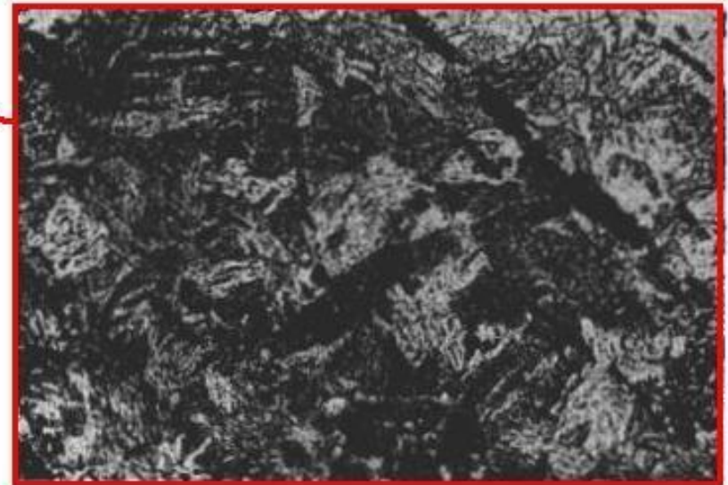
One of the dark-etching streaks (bainite)
