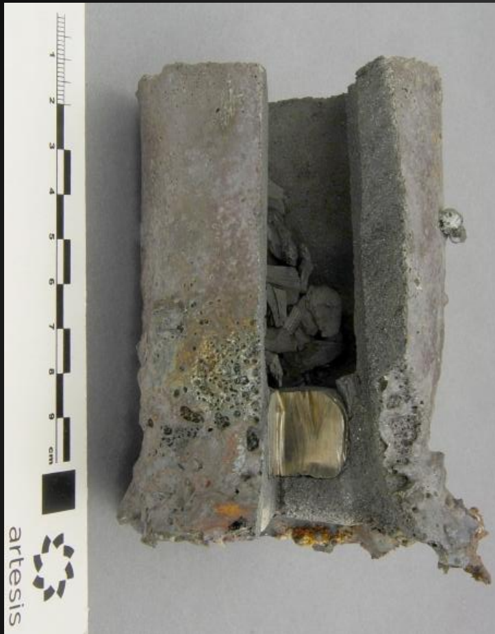
Crosssection of crucible after cooling
