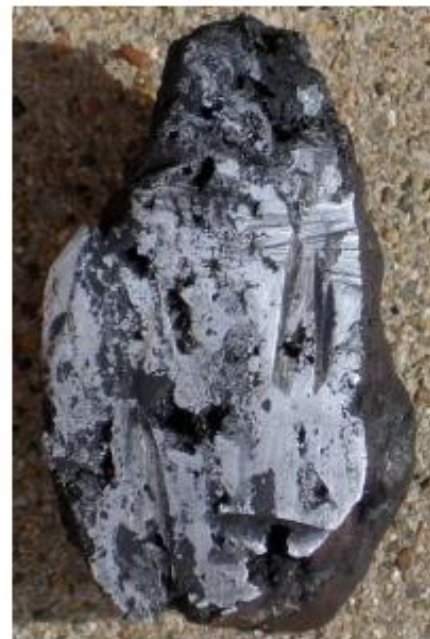
Figure 7- Bloom cross section
