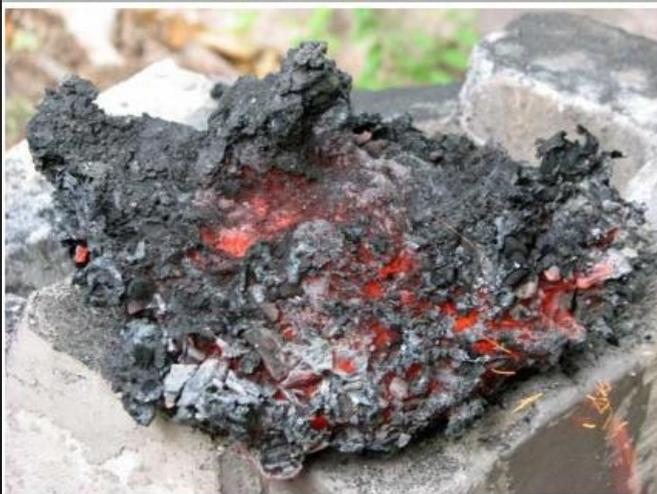
The bloom weighed at 2.5 kg right out of the forge, but after some hammering and cleaning, actually only contained about 1.125 kg of metal
