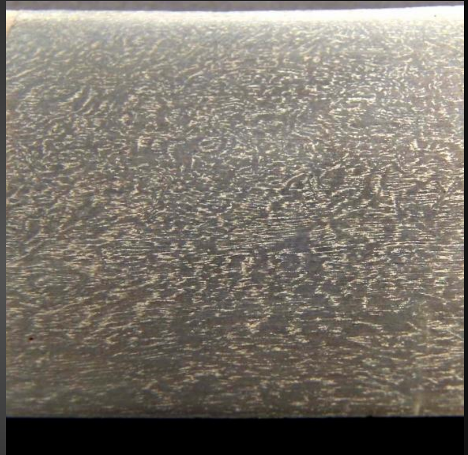
Polished and etched surface of a forged piece of crucible steel
