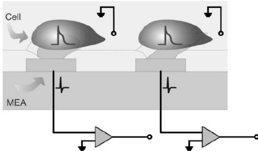
Figure 1.2 Schematic diagram of MEA for cell-based biosensors.
