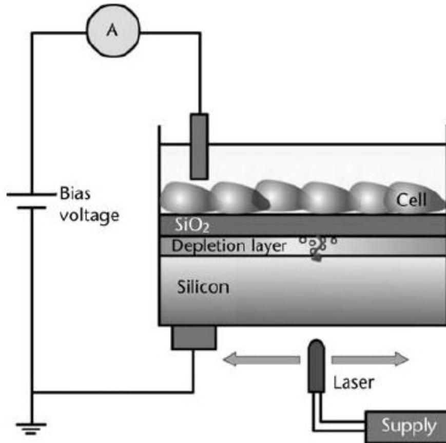
Figure 1.4 Schematic diagram of LAPS for cell-based biosensors.
