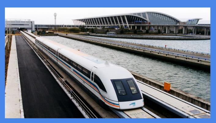
Maglev is a transport method that uses magnetic levitation to move vehicles without making contact with the ground.
