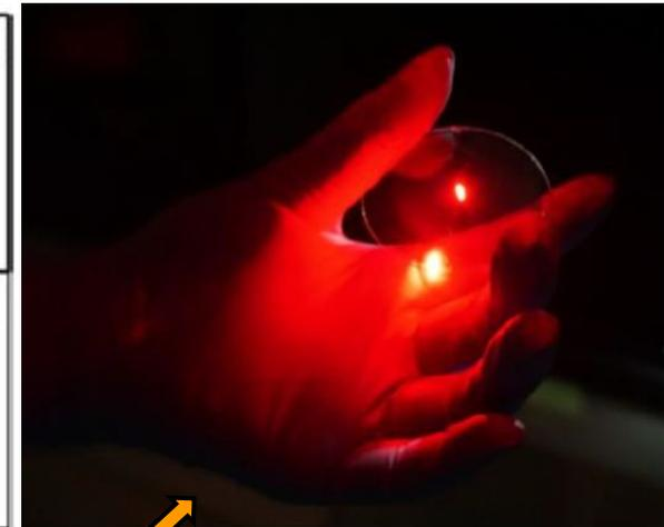
The picture of wafer-scale 8-layer GaSe film grown on mica. It is transparent and flexible.
