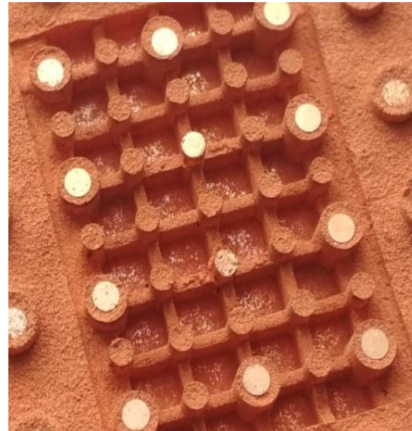
Vapor chamber with heterogeneous copper porous wick
