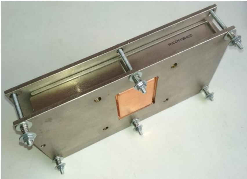
Vapor chamber with heterogeneous copper porous wick
