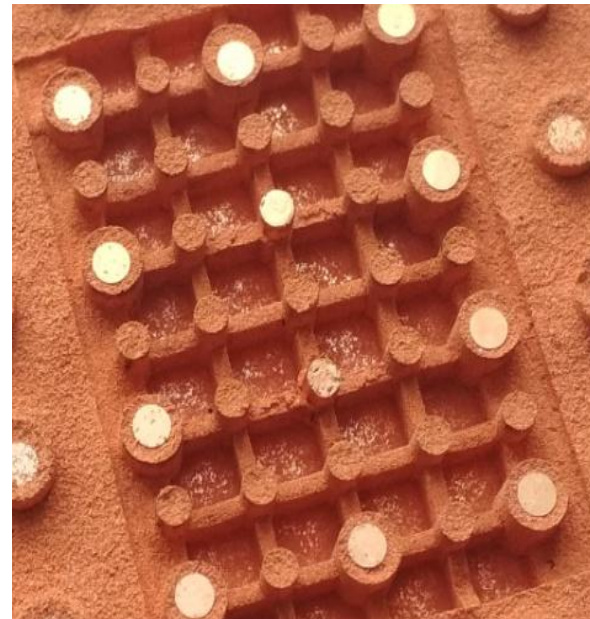
Vapor chamber with heterogeneous copper porous wick
