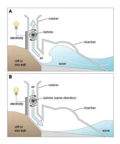
The two diagrams illustrate a method of creating electricity from the force of waves using a specifically designed man-made construction.
