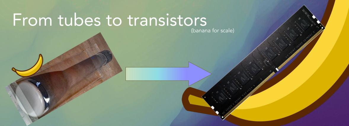
From using a Williams tube as a memory module, to multi-layered PCBs with millions of transistors on them it's clear that technology does not stand still
