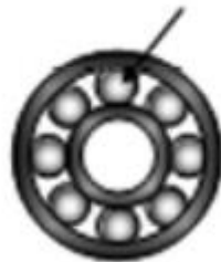
wear of rolling elements
