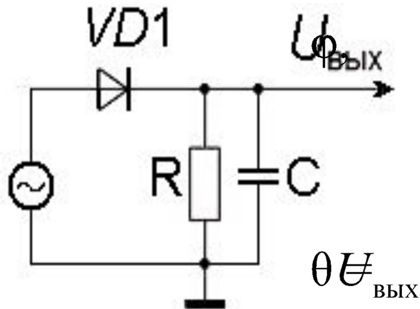
$$R \gg R_i, \quad \frac{1}{R \omega_0} \ll \frac{1}{RC \Omega}$$
