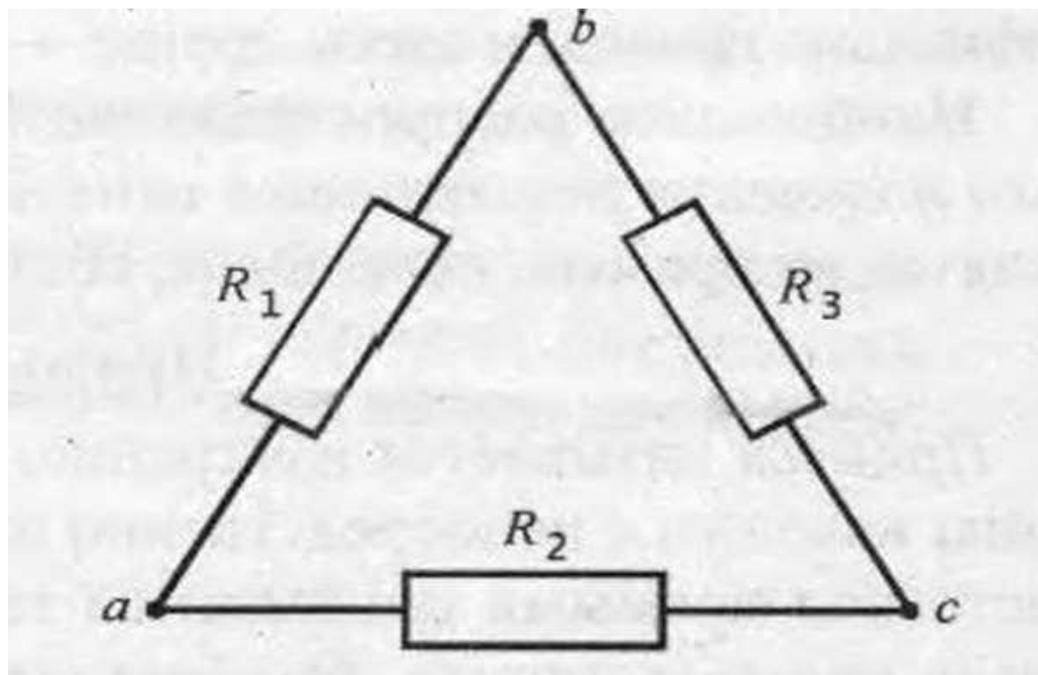
$$R_{ab} = \frac{R_1(R_2 + R_3)}{R_1 + R_2 + R_3}, \quad R_{ac} = \frac{R_2(R_1 + R_3)}{R_1 + R_2 + R_3}, \quad R_{bc} = \frac{R_3(R_1 + R_2)}{R_1 + R_2 + R_3}.$$
