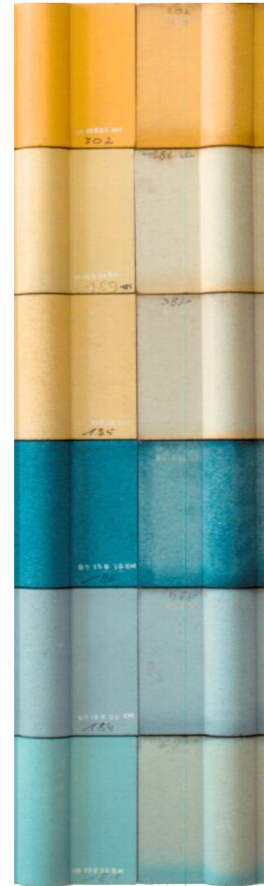
reference tile weathered sample tile
