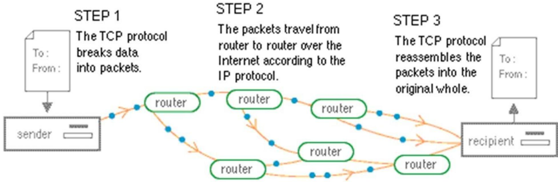
Figure 2. How data travels over the Net.
