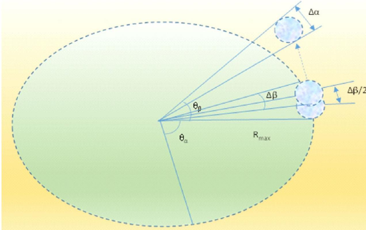
$$T_h = \frac{2\theta_\beta}{\Delta\beta} \frac{2\pi}{\Omega_\alpha}; \Omega_\alpha = \frac{\Delta\alpha}{NT_r} = \frac{\Delta\alpha F_r}{N} \Rightarrow T_h = \frac{4\pi\theta_\beta N}{\Delta\alpha\Delta\beta F_r}$$
