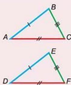
$$\left. \begin{array}{l} AB = DE \\ AC = DF \\ BC = EF \end{array} \right\} \Rightarrow$$
