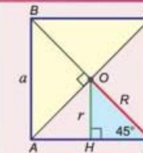
$$AC = a\sqrt{2}, \quad S_{ABCD} = a^2 \\ a = 2r, \quad R = r\sqrt{2}, \quad a = R\sqrt{2}$$
