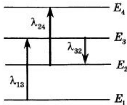
$$(N32) \quad \lambda_0 = 250 \text{ nm} \quad \left| \begin{array}{l} E_{\text{photon}} = E_n - E_k, \text{ vgl. } n > k \\ \frac{hc}{\lambda_{32}} = E_3 - E_2 \\ \frac{hc}{\lambda_{24}} = E_4 - E_2 \\ \frac{hc}{\lambda_0} = E_4 - E_1 \quad (\text{zu } f_{\text{min}} \text{ vgl. } \gamma_{\text{max}} \text{ u. } E_{\text{mean}}) \end{array} \right.$$
