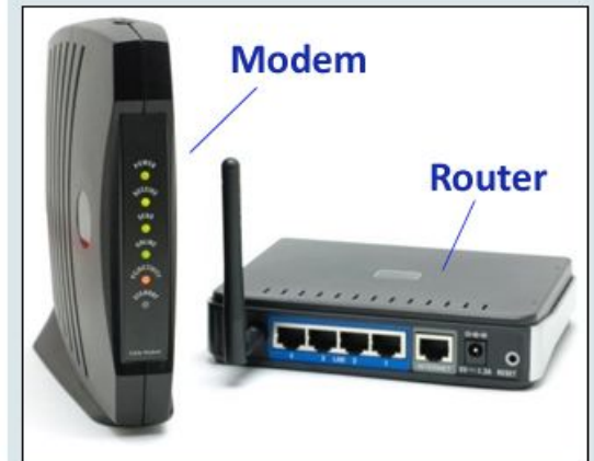
Some modems have routers built-in and some don't. If you want to connect multiple devices to the same internet connection you will need both.
