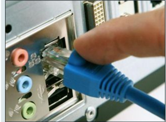
Network cables plug into the ports on network interface cards.
