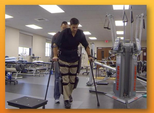
ReWalk is an exoskeleton — a set of electrically powered braces (подтяжки) that strap to the user's legs and use computers and motion sensors to control his movements
