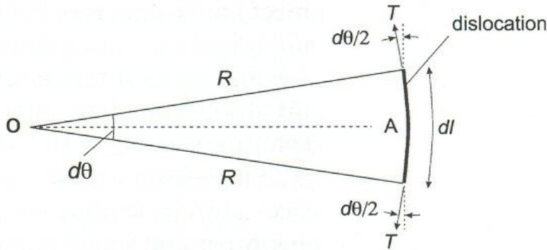
Figure 4.10 Curved element of dislocation under line tension forces  $T$ .
