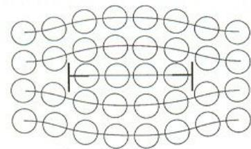
**Figure 3.18** Formation of a prismatic dislocation loop. (a) Represents a crystal with a large non-equilibrium concentration of vacancies. In (b) the vacancies have collected on a close-packed plane and in (c) the disc has
