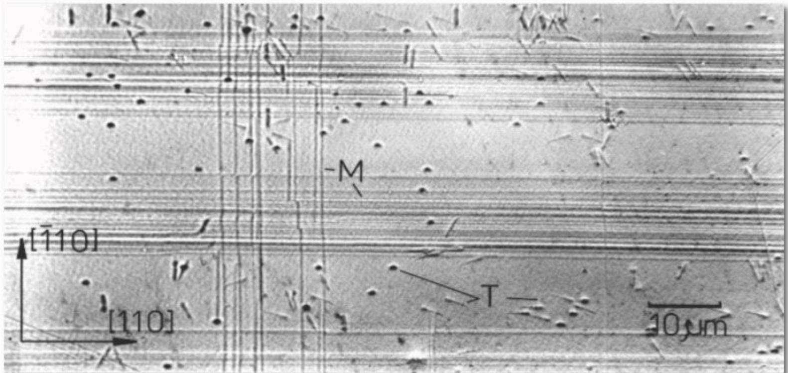
Etched misfit dislocations in epitaxial GaAs<sub>0.62</sub>P<sub>0.38</sub>/GaAs
