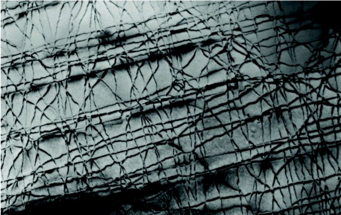
Misfit dislocations in (001) ZnSe/GaAs. MBE growth, layer thickness 495 nm. TEM bright field image.
