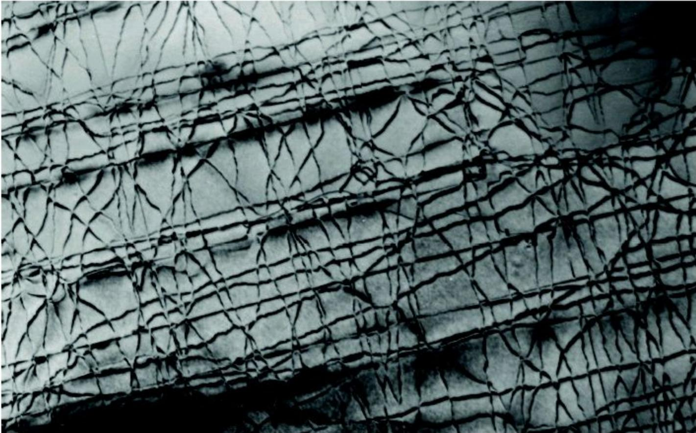
Misfit dislocations in (001) ZnSe/GaAs. MBE growth, layer thickness 495 nm.
