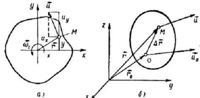
$$\vec{\omega} = \frac{1}{2} \begin{vmatrix} \vec{i} & \vec{j} & \vec{k} \\ \frac{\partial}{\partial x} & \frac{\partial}{\partial y} & \frac{\partial}{\partial z} \\ u_x & u_y & u_z \end{vmatrix} \Rightarrow \omega_y = \frac{1}{2} \left( \frac{\partial u_x}{\partial z} - \frac{\partial u_z}{\partial x} \right) \\ \omega_z = \frac{1}{2} \left( \frac{\partial u_y}{\partial x} - \frac{\partial u_x}{\partial y} \right)$$
