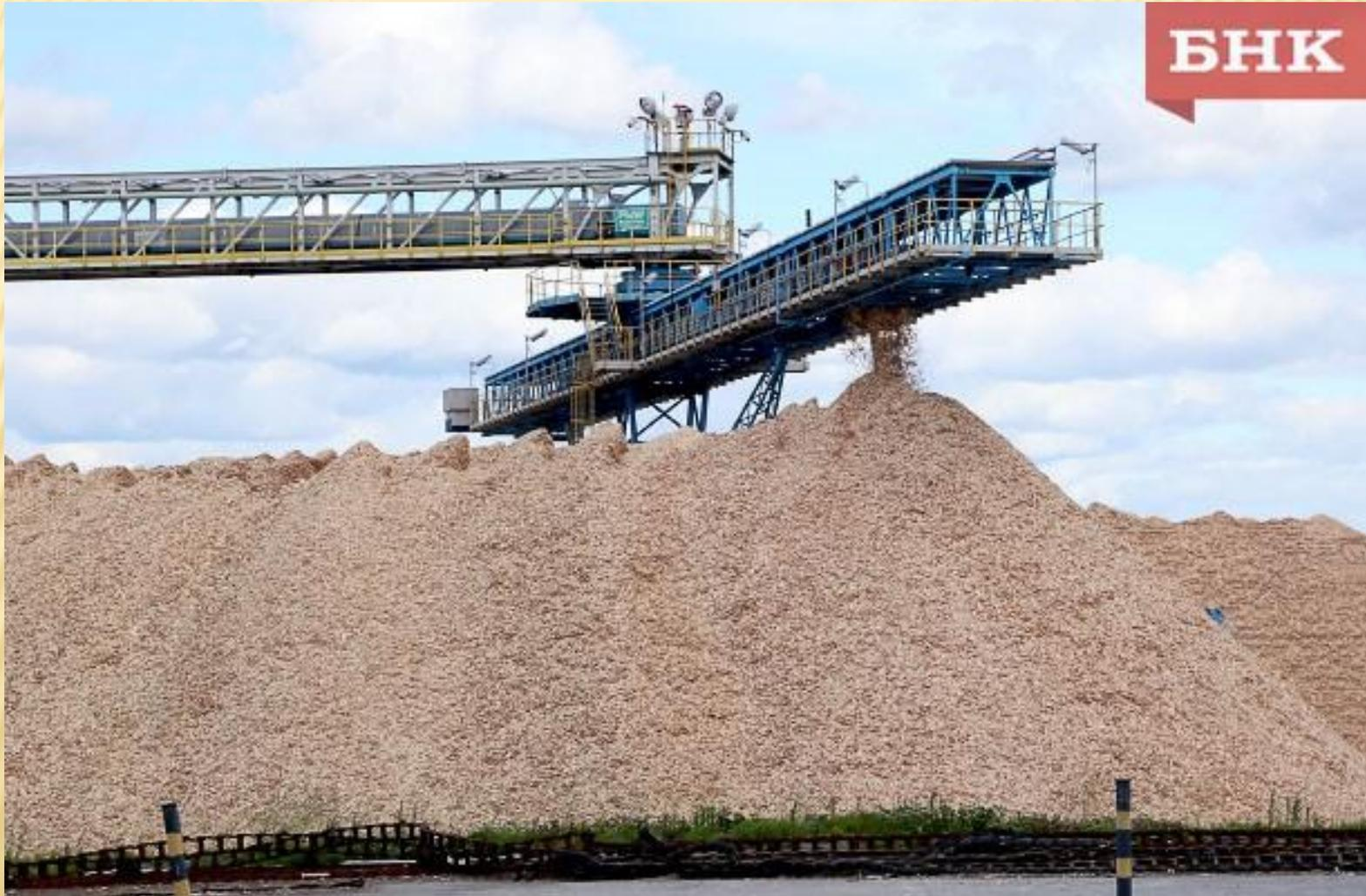
From a pile of chips is fed to sorting and forth on cooking
