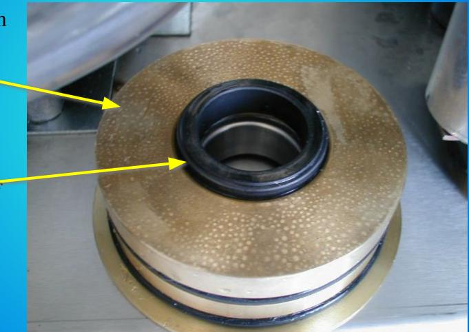
It is good practice to replace the water seal assembly, the two top and bottom bearings and the O rings any time the auger is removed.
