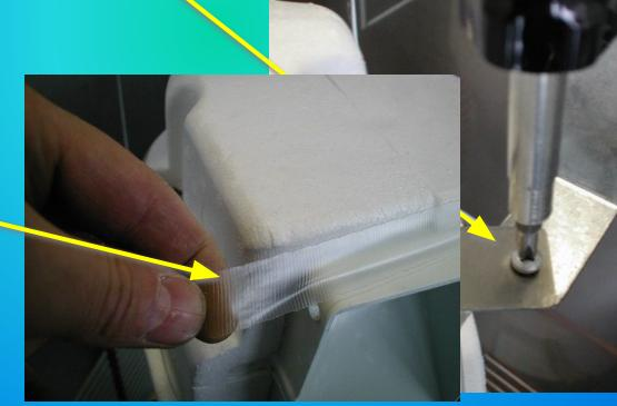
Remove from the plastic ice spout the two polystyre insulation covers then....
