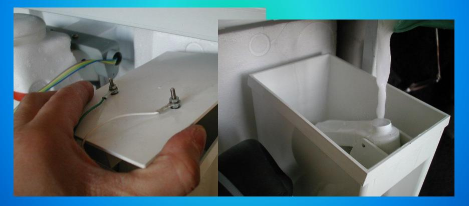
Leave the machine in **OFF** mode for approximately 20 minutes so to have the cleaning solution melting the scale into the entire water system.
