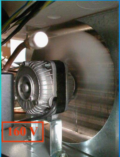
During normal operation mode the fan motor is energized at 230 V during its ON mode and....
