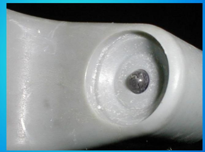
Check also for any possible accumulation of scale around the two holes located on the opposite sides of the ice chute.
