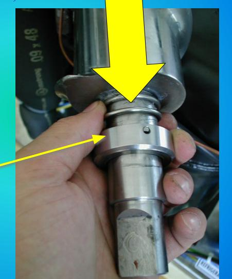
Unloose and remove the four bolts and lock-washers holding the freezer assembly to the aluminum adapter then
