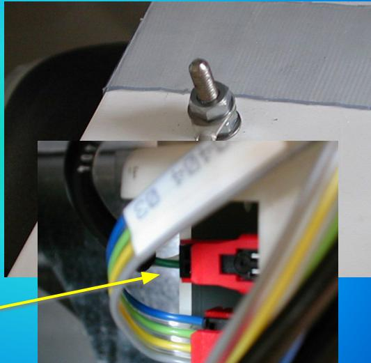
**ATTENTION.** The water level sensor operate by transmitting a low voltage current through the water. If water is very soft, with a very low content of mineral salts, no current is transmitting back to the PC Board tripping OFF the machine at <u>NO WATER LED.</u>
