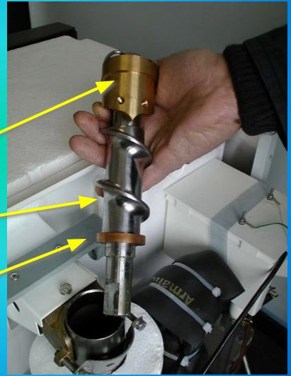
With a clip ring pliers remove the retaining ring and the cap from the ice breaker.
