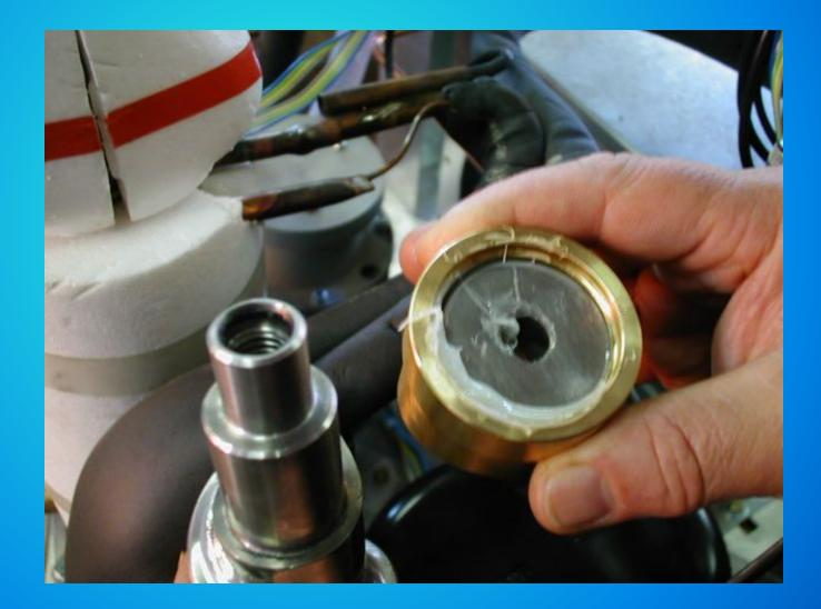
Clean away the old grease from the interior of the ice breaker and inspect the conditions of the top bearing
