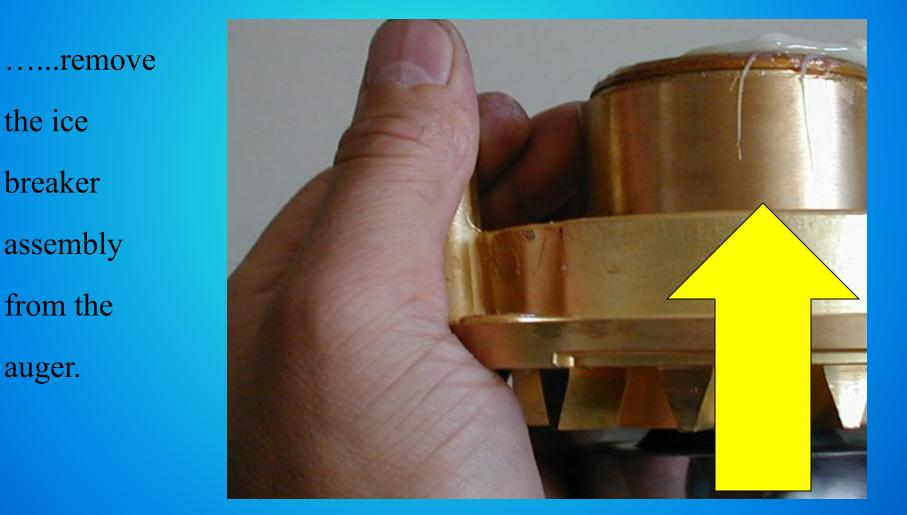
Clean away the old grease from the interior of the ice breaker and inspect the conditions of the top bearing
