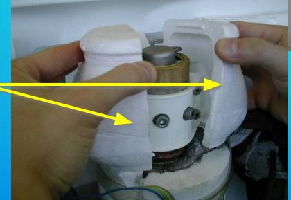
Unscrew and remove the two screws securing the brass ice breaker to the evaporator.
