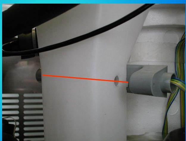
The two eyes placed on the opposite side of the plastic bracket must be perfectly clean with no dust and/or scale.
