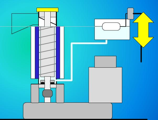
The unit frame is equipped by five series of holes so to secure at different level the water reservoir.
