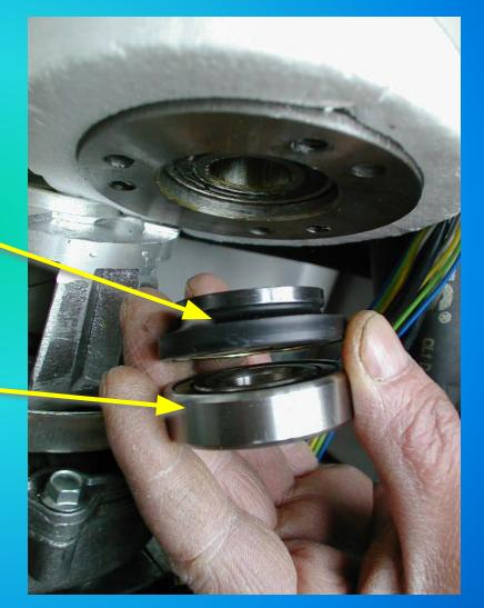
It is good practice to replace the water seal assembly, the two top and bottom bearings and the O ring any time the auger is removed.
