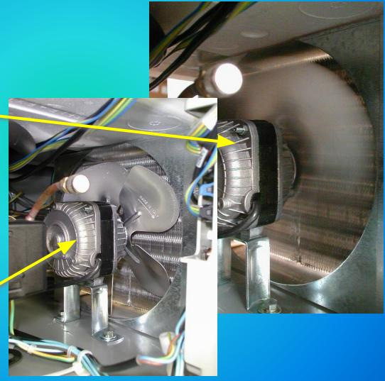
In case the power during the OFF mode is between 140 and 170 V the fan motor is keeping running but at lower speed that can cause an overheat of the same.
