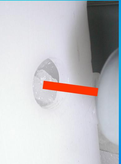
**ATTENTION.** The Optical Ice Level Control can be <u>affected by the sun light.</u> Avoid to leave the machine in operation directly under the sun light and/or without the service panels.
