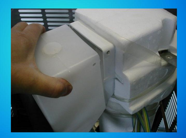
Unscrew the screw securing the ice spout metal bracket to the frame of the machine....
