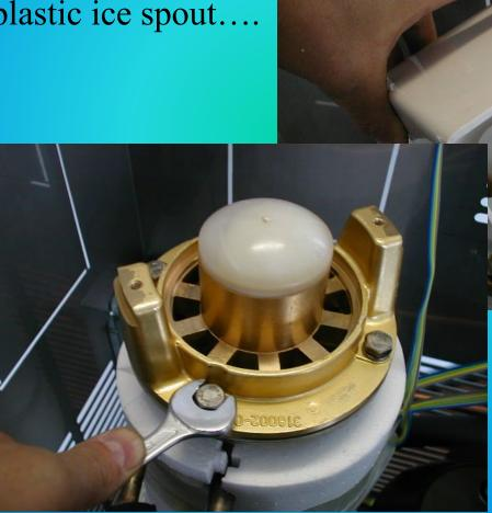
With a couple of screwdrivers rise up a little bit the ice breaker and auger assembly then ....
