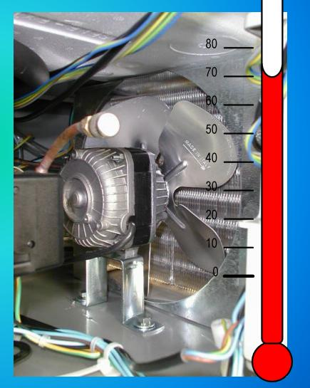
One more possibility (very rare) it is a faulty PC Board (TRIAC) that can keep energized the fan motor during the OFF period with a low voltage but higher then the minimum one need for tripping OFF the motor.
