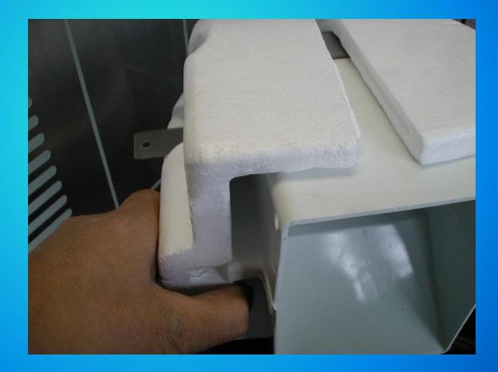
....unloose the two screws securing the ice spout metal bracket to the ice breaker....
