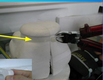
.....two polystyrene insulation from the spout.
