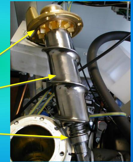
With a screwdriver remove the plastic cap from the upper side of the ice breaker.
