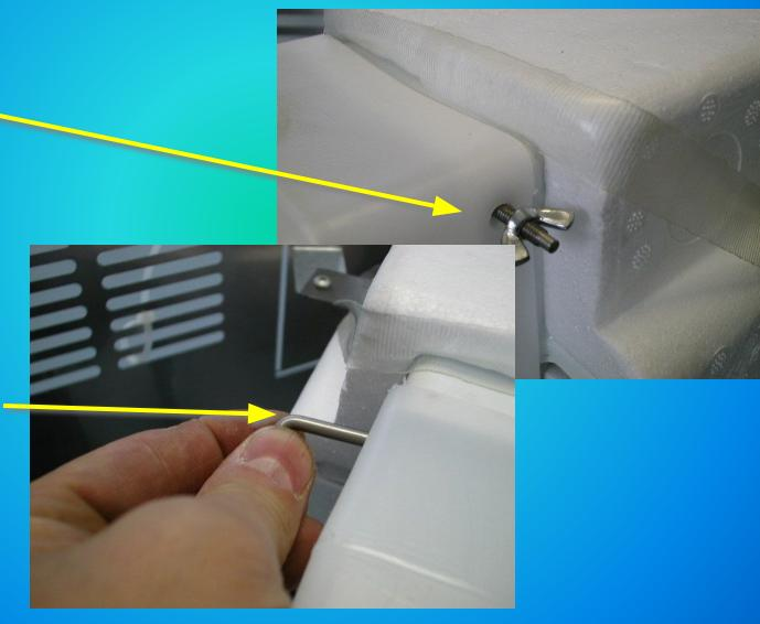
Remove the ice chute with the optical ice level control secured on it then....
