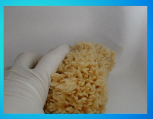
**REMEMBER.** To prevent the accumulation of undesirable bacteria it is necessary to sanitize the interior of the storage bin with a sanitizing solution every week.
