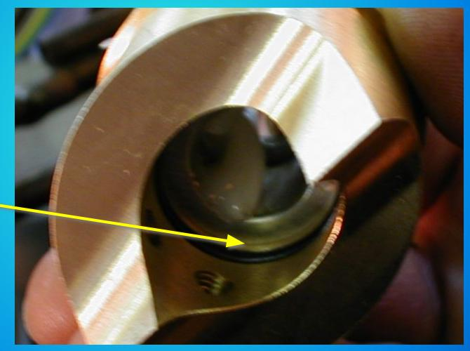
Slide off from the bottom of the auger the upper half of the water seal.
