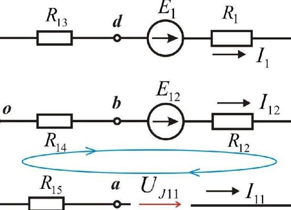
$$I_{12} \cdot R_{14} + I_{12} \cdot R_{12} - U_{J11} - I_{11} \cdot R_{15} = E_{12}$$
