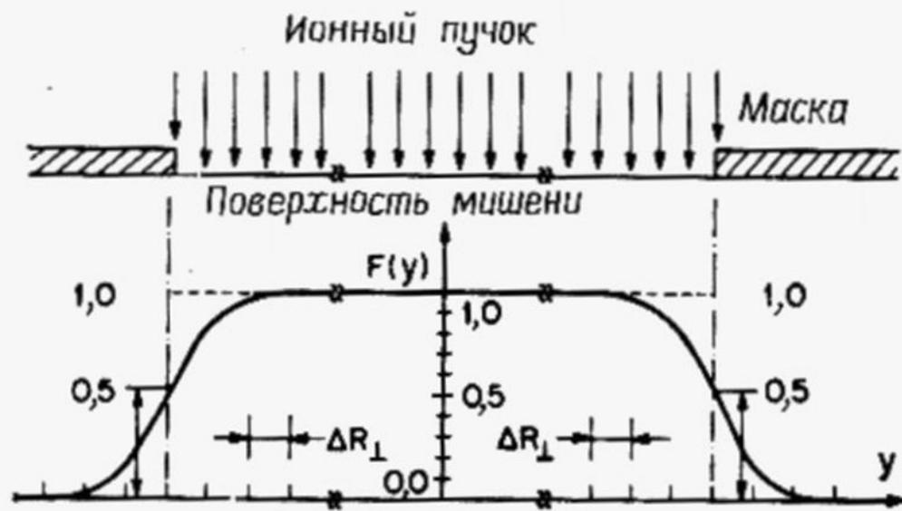
$$N(x, y) = \frac{N(x)}{2} \left[ \operatorname{erfc} \left( \frac{y-a}{\sqrt{2} \cdot \Delta R_{\perp}} \right) - \operatorname{erfc} \left( \frac{y+a}{\sqrt{2} \cdot \Delta R_{\perp}} \right) \right]$$
