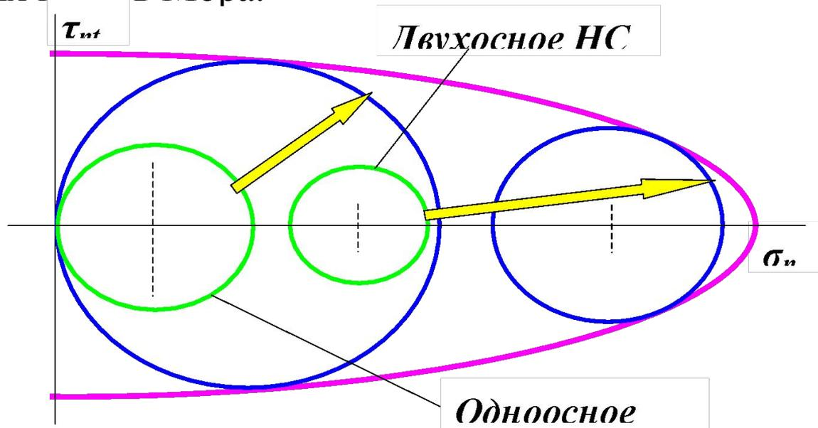
$$\sigma_{\text{экв}}^M = \sigma_1 - \frac{[\sigma_p]}{[\sigma_c]} \sigma_3 \quad \sigma_{\text{экв}}^M \leq [\sigma_p]$$
