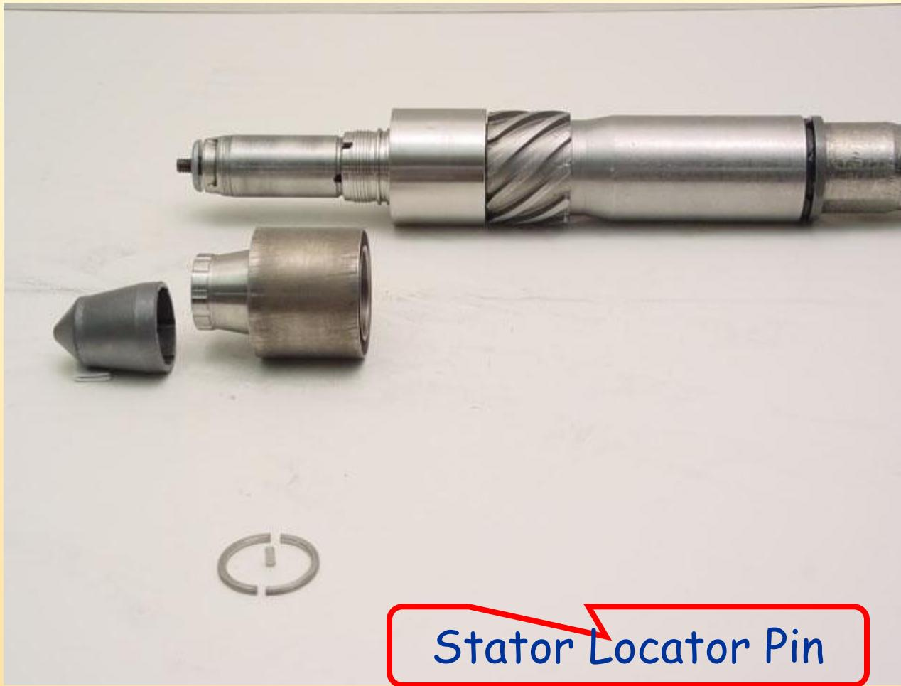
Stator Locator Pin
