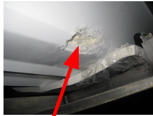
Big damage of hull
