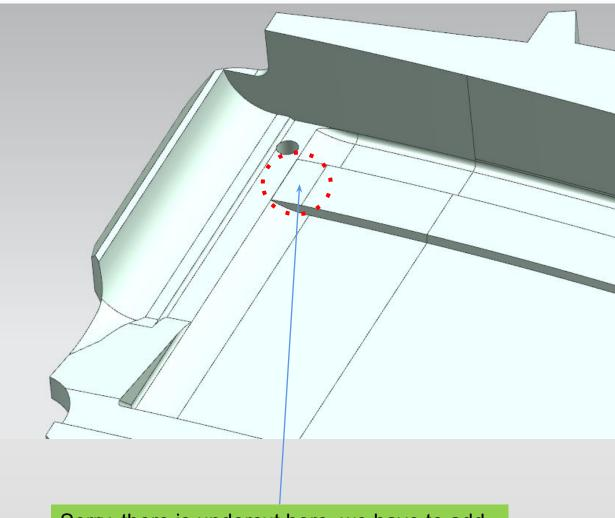
Sorry, there is undercut here, we have to add a little material here to remove the undercut, otherwise the part can not be released from the slide. Thank you.
