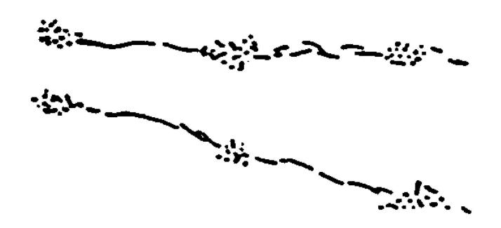
**Pittings** which are close together or form a linear pattern can signify crack formation beneath the surface. Such pittings should be investigated by a materials expert.
