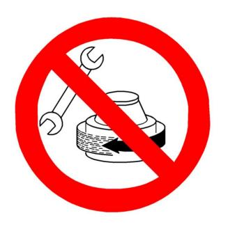
Do not loosen any part and do not carry out maintenance or repair on the separator before the separator is at a standstill!
