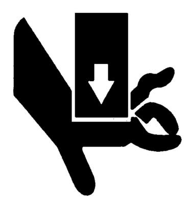
When transporting and assembling machine parts, avoid crushing and shear strain.
