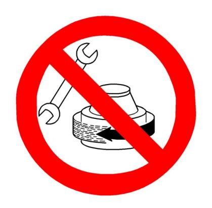
Do not loosen any part and do not carry out maintenance or repair work on the separator before the separator is at a standstill!
