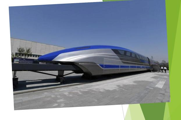
Maglev is a system of train transportation that uses two sets of electromagnets With maglev technology, the train travels along a guideway of electromagnets which control the train's stability and speed
