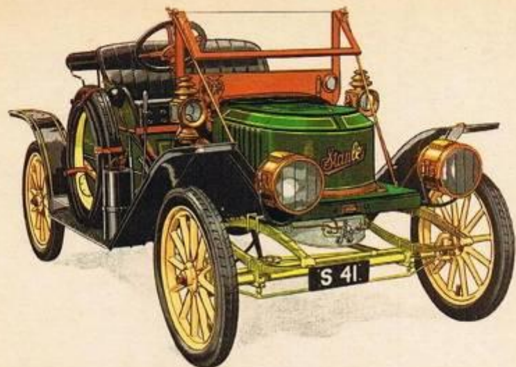
1911 10 h.p. STANLEY STEAM CAR Model 52 with Runabout body. Engine, two cylinder double acting simple expansion;
