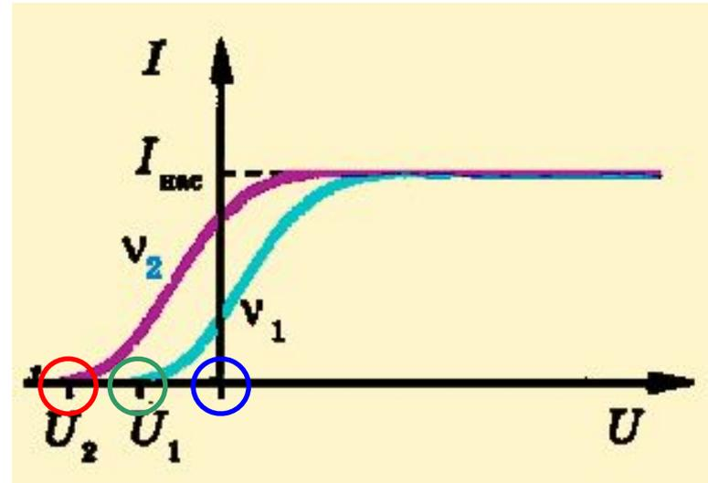
$$\left\{ \begin{array}{l} eU_{31} = \frac{m v_{\text{max}1}^2}{2} \\ eU_2 = \frac{m v_{\text{max}2}^2}{2} \end{array} \right.$$
