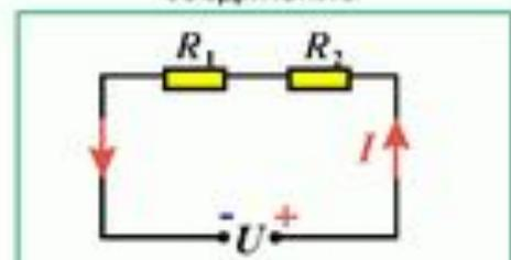
$$\left. \begin{aligned} Q_1 &= IR_1^2 t \\ Q_2 &= IR_2^2 t \end{aligned} \right\} \frac{Q_1}{Q_2} = \frac{R_1}{R_2}$$
