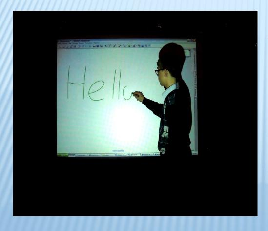
We can use it to write a text or to draw in different colors on the SMART Board, Most models of SMART Board include a pen tray on the front of the interactive whiteboard that holds four plastic pen tools and an eraser
