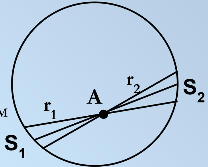
$$E = \frac{q_1}{4\pi\epsilon_0 r_1^2} - \frac{q_2}{4\pi\epsilon_0 r_2^2} = \frac{\sigma}{4\pi\epsilon_0} \left( \frac{S_1}{r_1^2} - \frac{S_2}{r_2^2} \right) = 0$$
