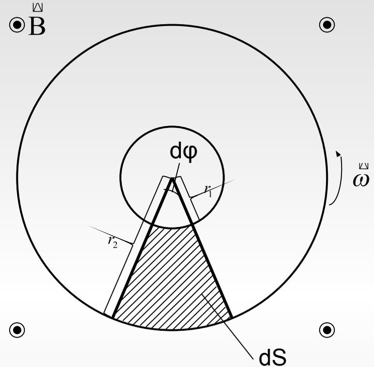
$$E = \frac{1}{2} \omega B (r_2^2 - r_1^2)$$
