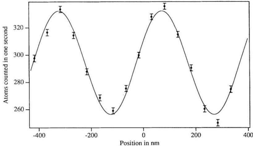
FIG. 4. Interference signal from 400 s of data ( $\sim 23$  s per point). Background hot-wire noise of 40 counts/s subtracted. The solid line is a least-squares fit by a sine function with 400-nm period. Error bars are 1 standard deviation assuming Poissonian noise, and slightly underestimate the noise because of the super-Poissonian character of the hot-wire background.
