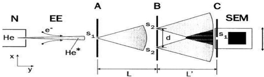
FIG. 2. Schematic representation of the experimental setup: nozzle system and gas reservoir N; electron impact excitation EE; entrance slit A, double slit B, and detector screen C; secondary electron multiplier SEM (mounted together with C on a translation stage). Dimensions:  $d = 8 \mu\text{m}$ ,  $L = L' = 64 \text{ cm}$ ; slit widths:  $s_1 = 2 \mu\text{m}$ ,  $s_2 = 1 \mu\text{m}$ .
