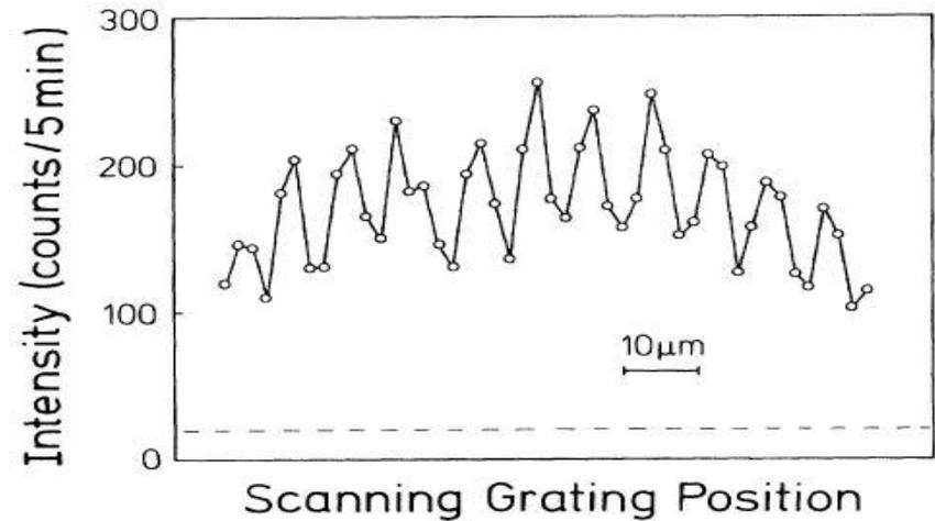
FIG. 5. Atomic density profile, monitored with the  $8\text{-}\mu\text{m}$  grating in the detector plane, as a function of the lateral grating displacement. The dashed line is the detector background. The line connecting the experimental points is a guide to the eye.
