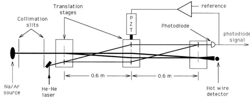
FIG. 1. A schematic of our interferometer showing the active vibration isolation system. Not to scale. The  $0.4\text{-}\mu\text{m}$ -period atom gratings are indicated by a vertical dashed line, and the  $3.3\text{-}\mu\text{m}$ -period optical gratings by a vertical solid line.
