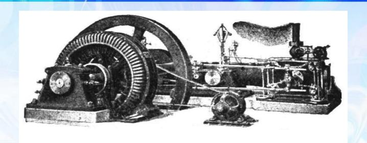
The Dynamo was the first electrical generator capable of delivering power for industry. The dynamo uses electromagnetic principles to convert mechanical rotation into a pulsing direct electric current through the use of a commutator. A dynamo machine consists of a stationary structure, which provides a constant magnetic field, and a set of rotating windings which turn within that field.
