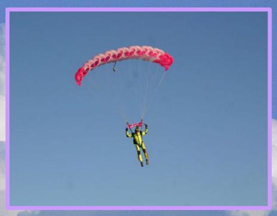
There are two kinds of parachutes: parachute with a round dome (*round parachute*) and parachute with rectangular gliding dome (*parachute-wing*).
