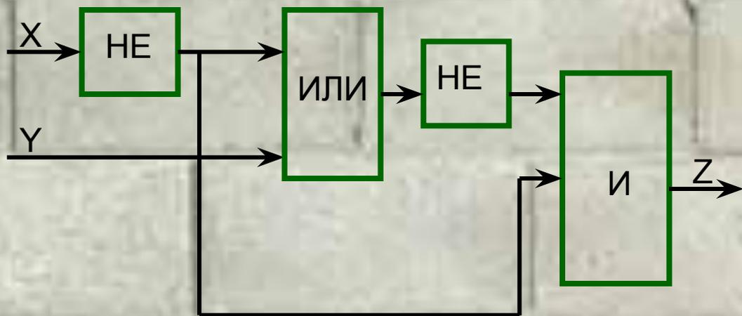
$$Z = \overline{X} \& Y \vee \overline{\overline{X}}$$
