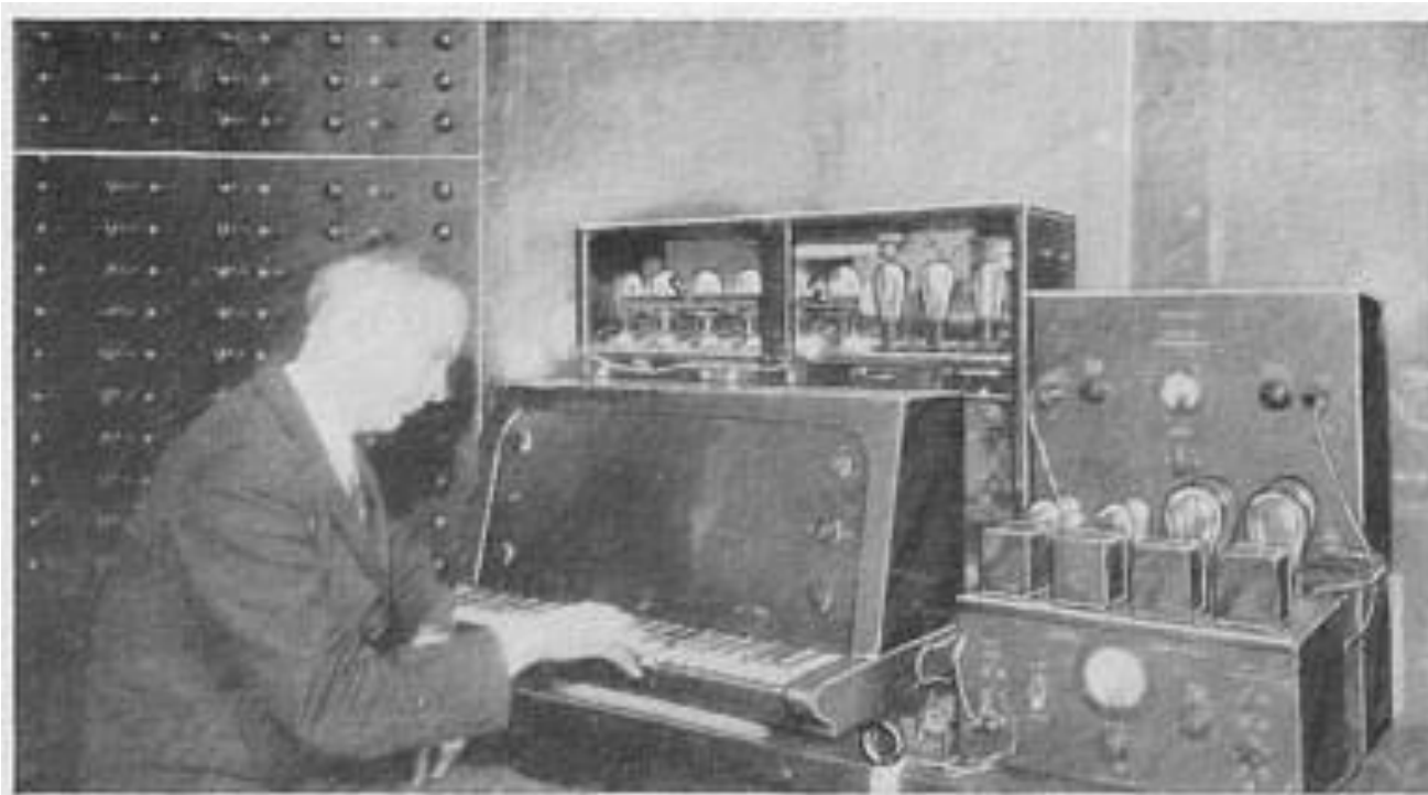
Shown above is an electric organ in the laboratories of the Westinghouse Electric & Manufacturing Company. It is energized by vacuum tubes. Mr. R. C. Hitchcock is seen seated at the console; at his left is the large control panel
