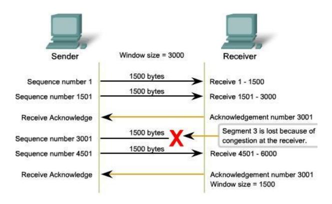
If segments are lost because of congestion, the Receiver will acknowledge the last received sequential segment and reply with a reduced window size.
