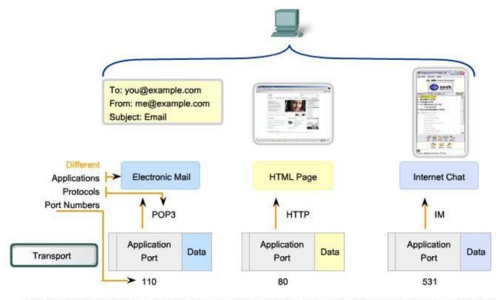
Data for different applications is directed to the correct application because each application has a unique port number.
