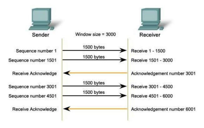
The window size determines the number of bytes sent before an acknowledgment is expected.
