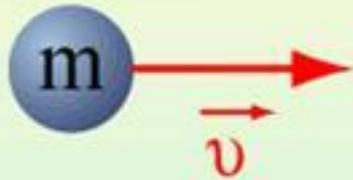
$$\vec{v} = \text{const}, \\ \text{при } \vec{F} = 0$$
