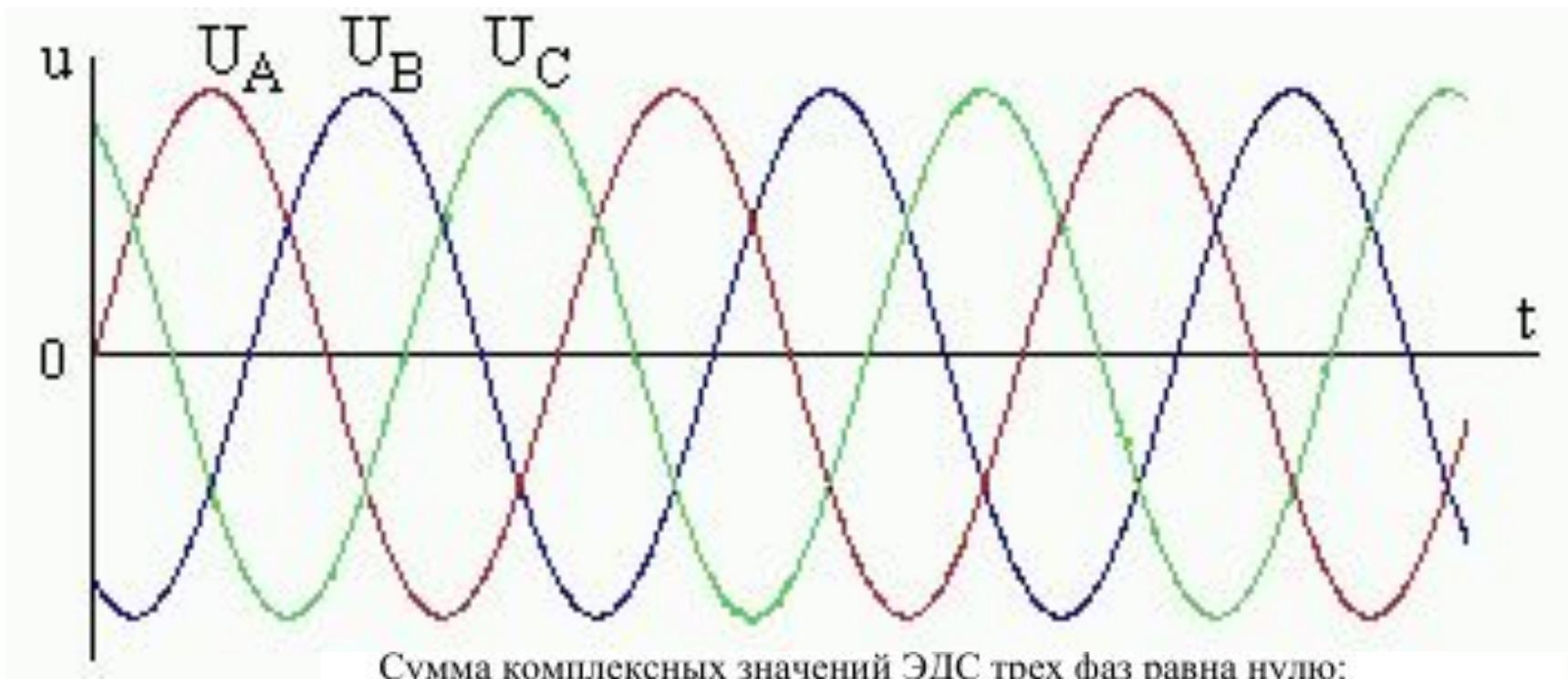
$$\dot{E}_A + \dot{E}_B + \dot{E}_C = E + Ee^{-j120^\circ} + Ee^{+j120^\circ} = E - \frac{E}{2} - j\frac{\sqrt{3}}{2}E - \frac{E}{2} + j\frac{\sqrt{3}}{2}E = 0.$$
