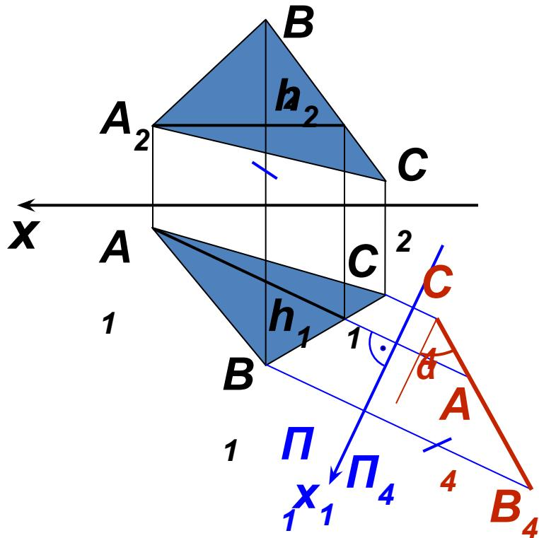
$$\begin{aligned}1. \quad & \Pi_4 \perp \Pi_1 \\& \Pi_4 \perp h \in \Sigma \\& (\Delta ABC)\end{aligned}$$
