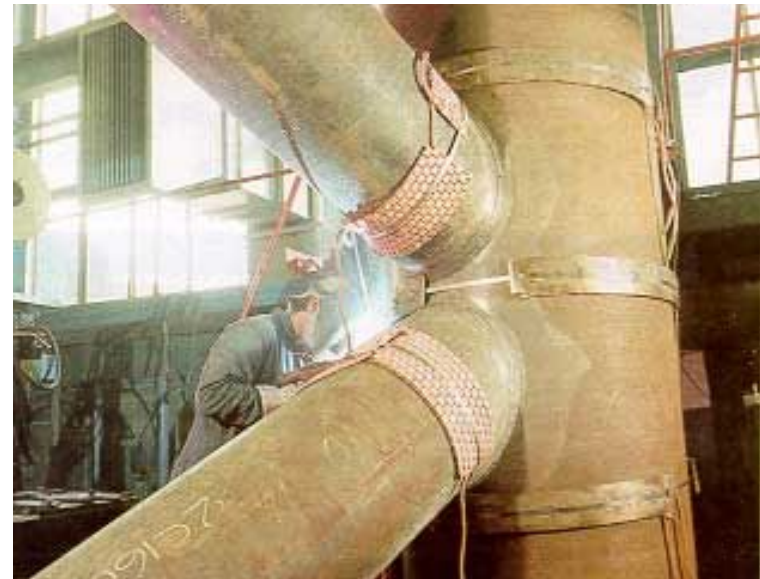
Preheating to avoid hydrogen cracking
