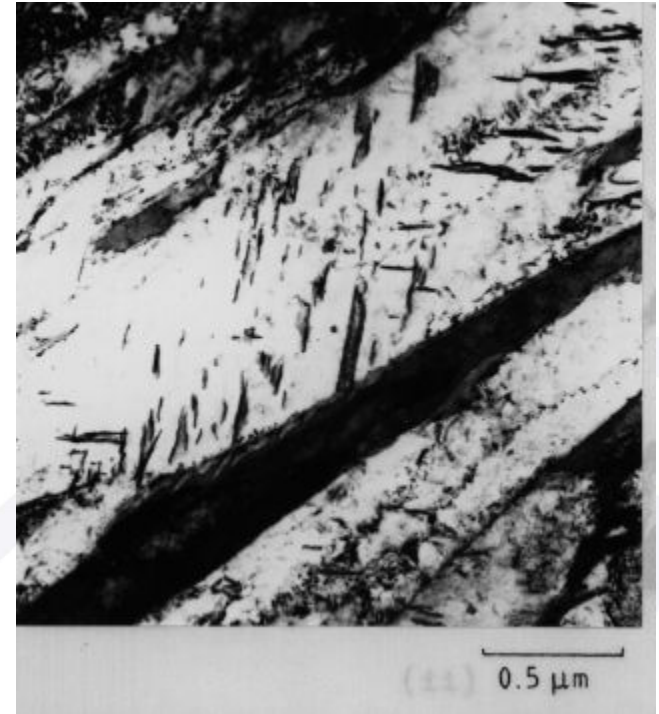
Micrography of cementite (intermetallic) in lower bainite
