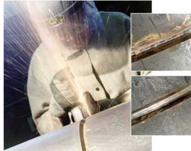
Prevention by grinding between runs
