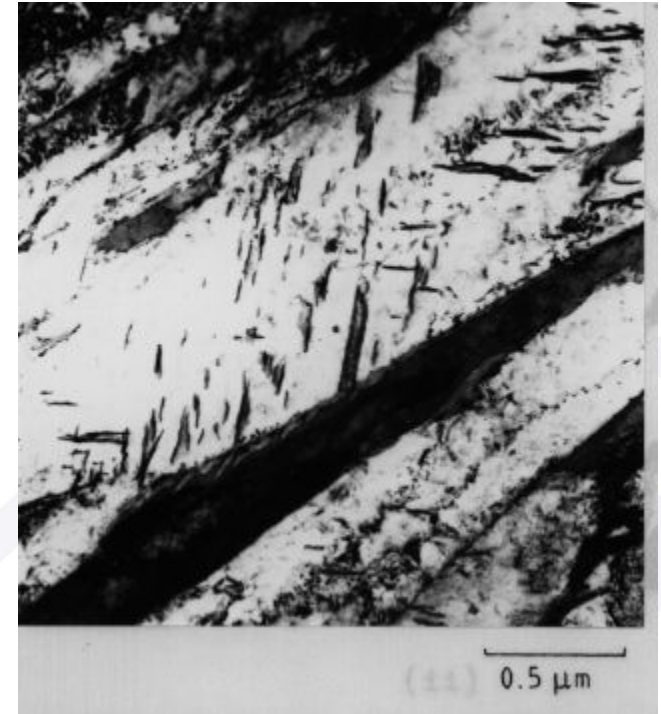
Micrography of cementite (intermetallic) in lower bainite
