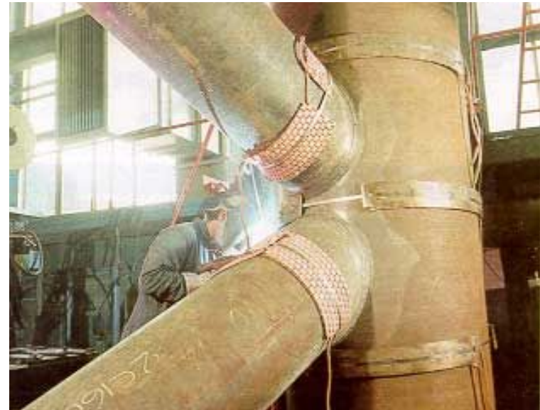
Preheating to avoid hydrogen cracking
