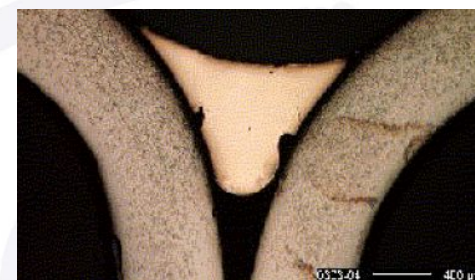
Braze welding between C-steel and aluminium alloy with ZnAl14 alloy P = 1.1 \text{ kW} , v = 1,0 \text{ m/min}
