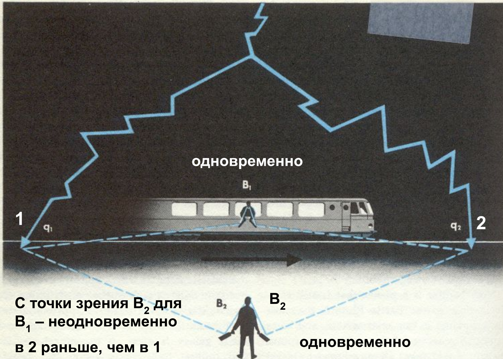
A stationary observer B_2 on the railway embankment sees the forked lightning strike at two positions q_1 and q_2 simultaneously. The observer B_1 moving with the train undergoing uniform rectilinear motion, sees the lightning strike q_2 a fraction of a second before q_1 . The reason for this is the finite signal speed of light.
